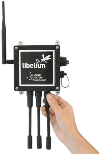
Figure: Connecting a sensor probe to Wasmote Plug & Sense!
