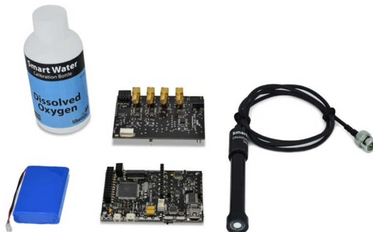
Figure: Image of the material necessary for the dissolved oxygen calibration process
