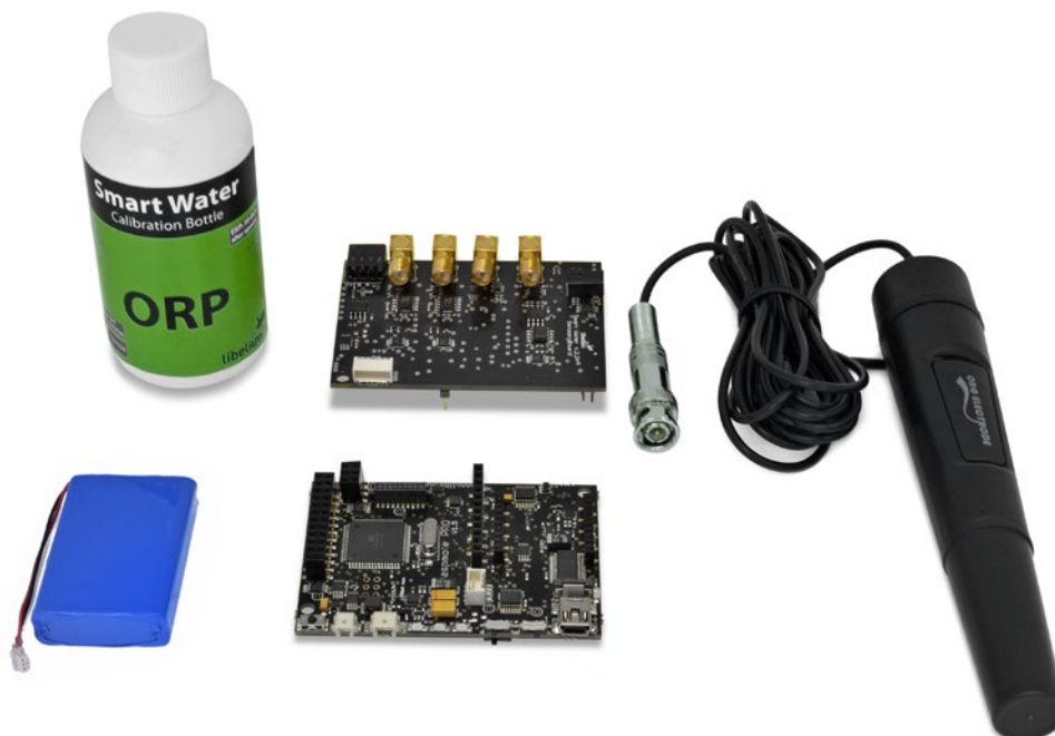
Figure: Image of the material necessary for the ORP calibration process
