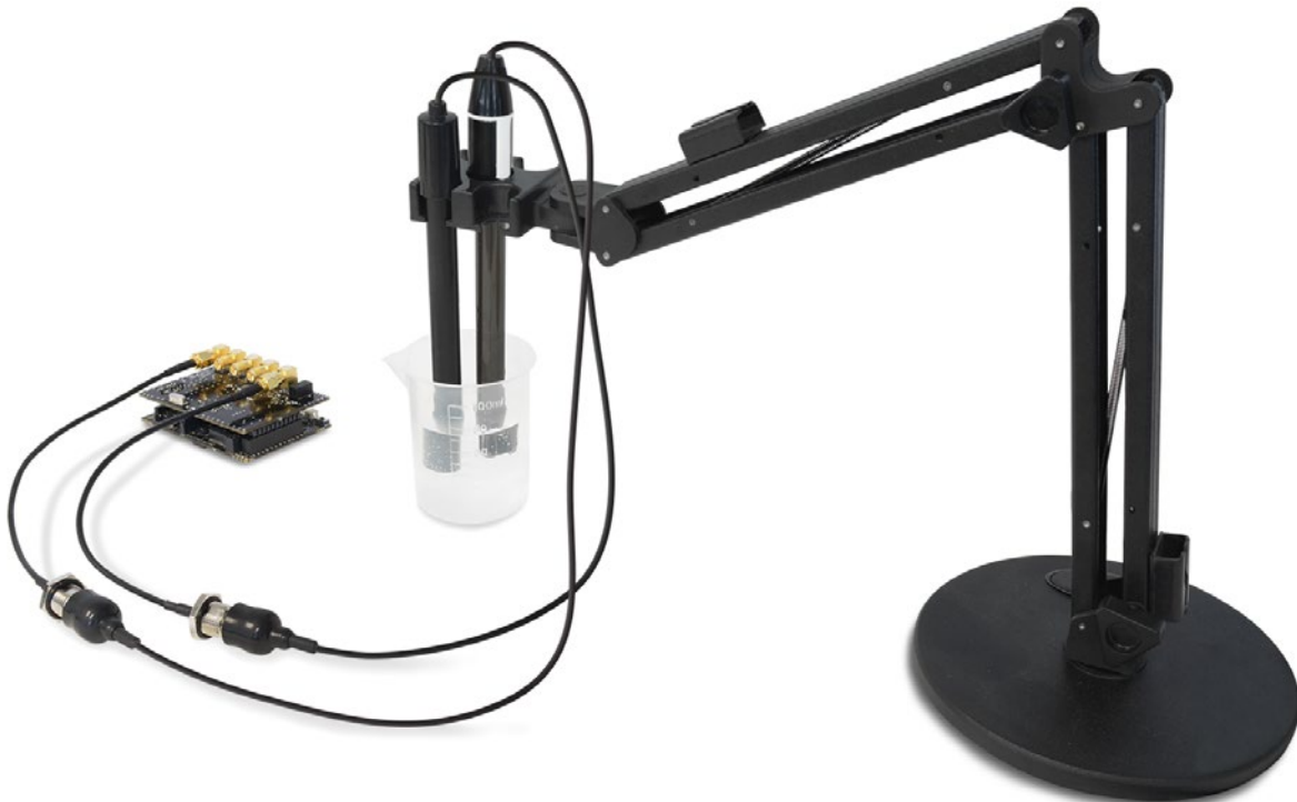
Figure: Calcium Ion ( \text{Ca}^{2+} ) Sensor Probe in 10 mg/L solution
