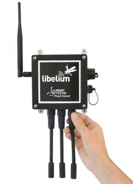
Figure: Connecting a sensor probe to Waspote Plug & Sense!
