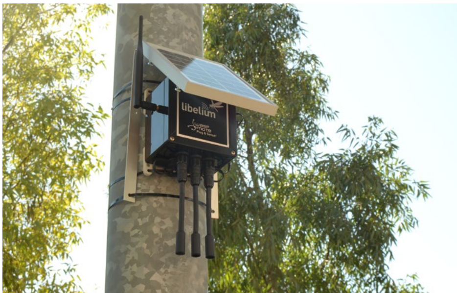
Figure: Wasp mote Plug & Sense! powered by an external solar panel
