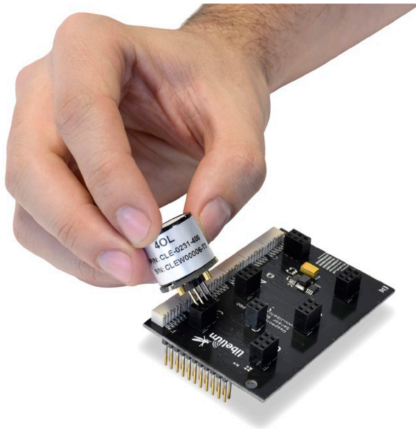
Figure: Connection of a 3-electrode AFE board
