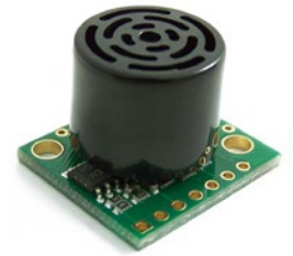
Figure: Ultrasonic I2CXL-MaxSonar®- MB1202 from MaxBotix™ Sensor
