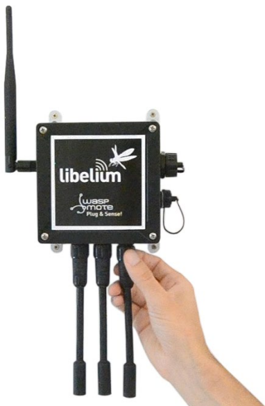
Figure: Connecting a sensor probe to Wasp mote Plug & Sense!
