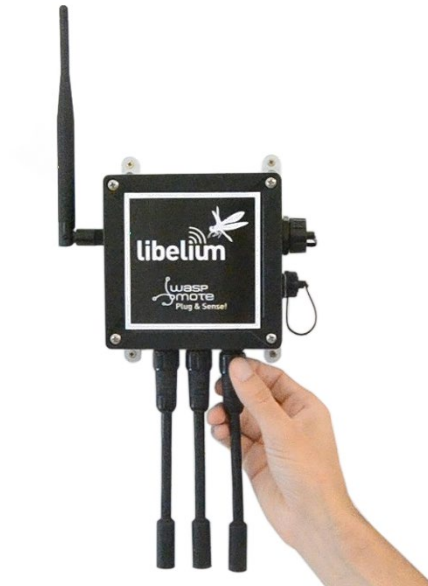
Figure: Connecting a sensor probe to Wasp mote Plug & Sense!
