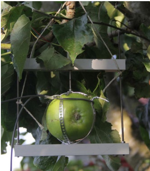
Figure: Ecomatik DF sensor with apple
