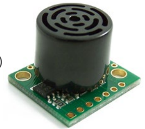
Figure: Ultrasonic I2CXL-MaxSonar®-MB1202 from MaxBotix™ sensor
